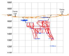
Areas where sinkholes were probable were characterized by: depth to opening of 100-ft or less (Crown Pillar thickness of 100-ft or less); orebody width of 100-ft or more; and Stopes that were vertically extensive. Potentially sinkhole areas were identified on a surface plan and fenced by the Cleanup Contractor.
